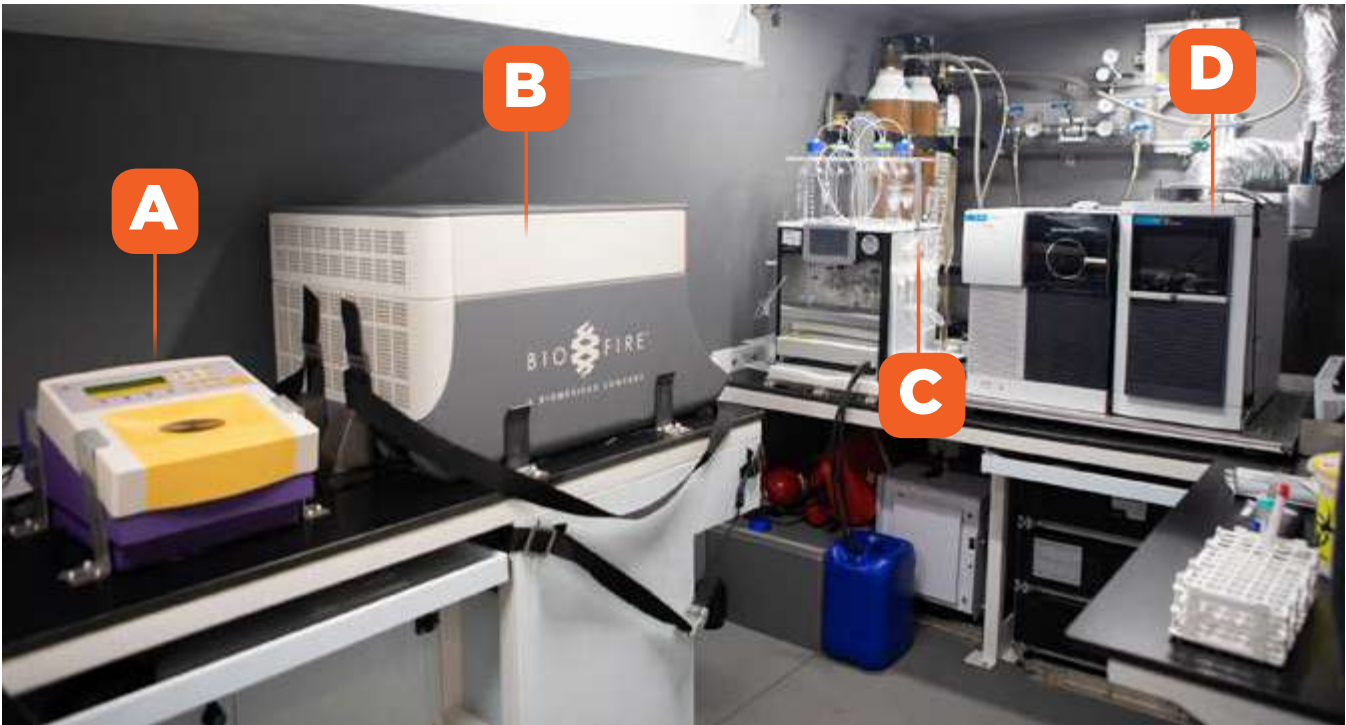
▲ The interior of the Mobile Lab is equipped with multidisciplinary capabilities for rapid detection of radionuclides, common foodborne pathogens as well as pesticides and residues using a (A) gamma spectrometer, (B) multiplex PCR machine, (C) automated solid phase extraction (SPE) clean-up system and (D) gas chromatography–tandem mass spectrometry (GC-MS/MS System) respectively. Having these equipment readily available in the Mobile Lab supports SFA’s special operations such as the investigation of illegal imports of undeclared high-risk fruits and vegetables. It also allows SFA to take immediate enforcement action, which could serve as an effective deterrent against such errant behaviour.
