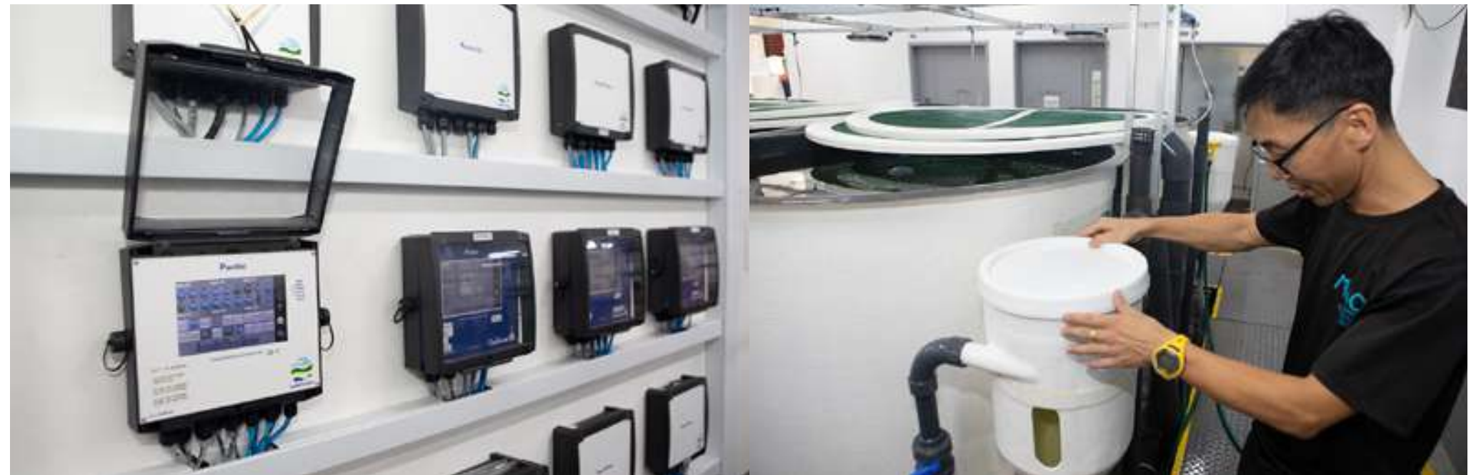
↑ The RAS is equipped with various accessories such as dissolved oxygen sensors, fish faecal collection unit, and water chiller to enable a variety of trials with different species and conditions.
