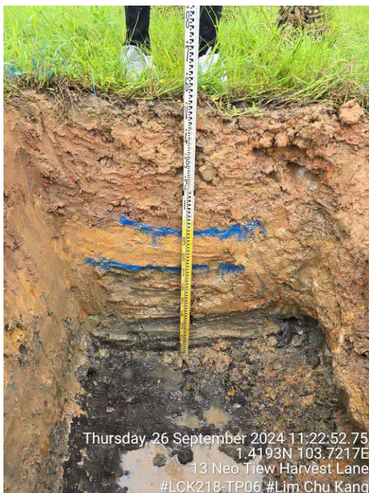
Figure 3.24 Closeup View of Trial Pit LCK218-TP06
