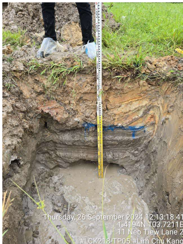
Figure 3.20 Closeup View of Trial Pit LCK218-TP05
